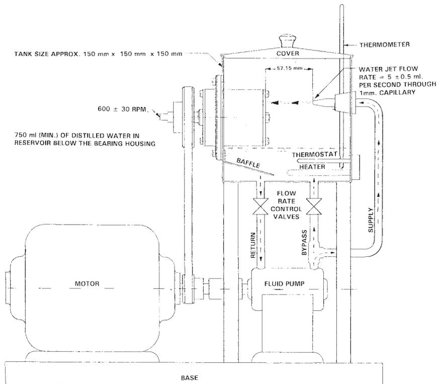
FIG. 1 Water Washout Characteristics of Lubricating Grease Apparatus
