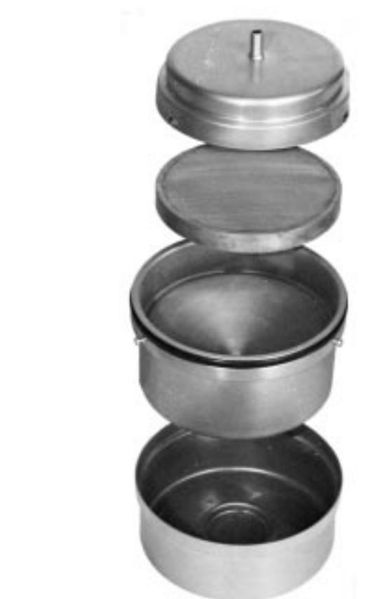
FIG. 1 Pressure Bleeding Test Cell A
