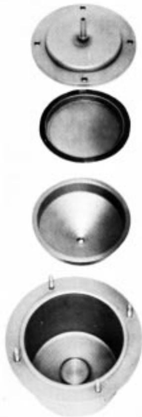
FIG. 5 Pressure Bleeding Test Cell C
