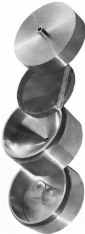
FIG. 3 Pressure Bleeding Test Cell B
