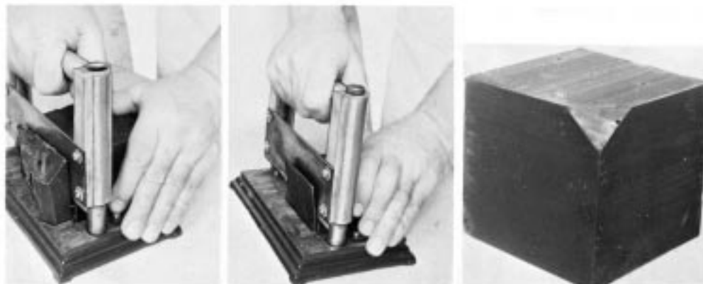
FIG. 3 Preparing Block Sample for Penetration Measurement
