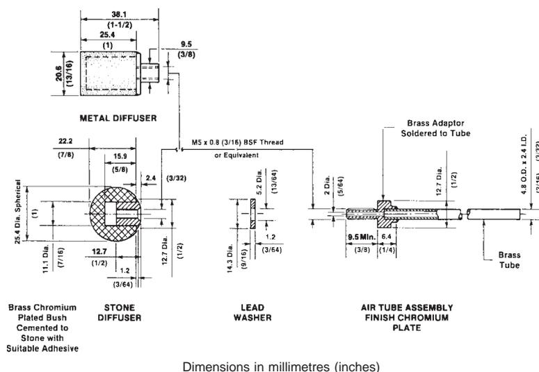
FIG. 2 Attachment of Gas Diffusers to Air-Inlet Tubes
